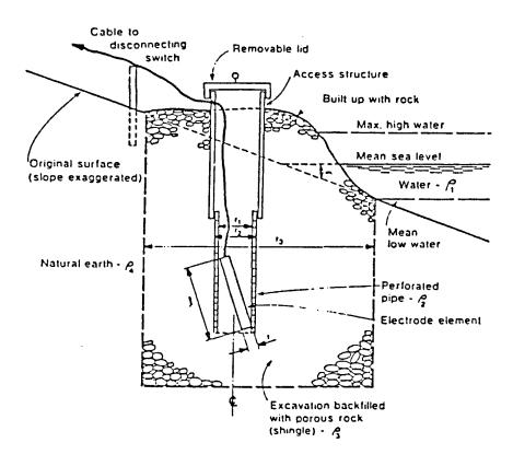
FIGURE 1. Diagrammatic section through hypothetical shore electrode.
