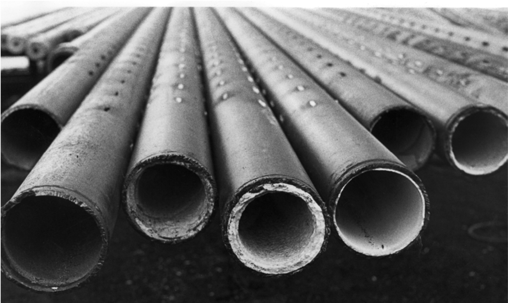
Figure 8.1: Calcite scaling inside liner – note plugged slots (Thorhallsson, 2003).
