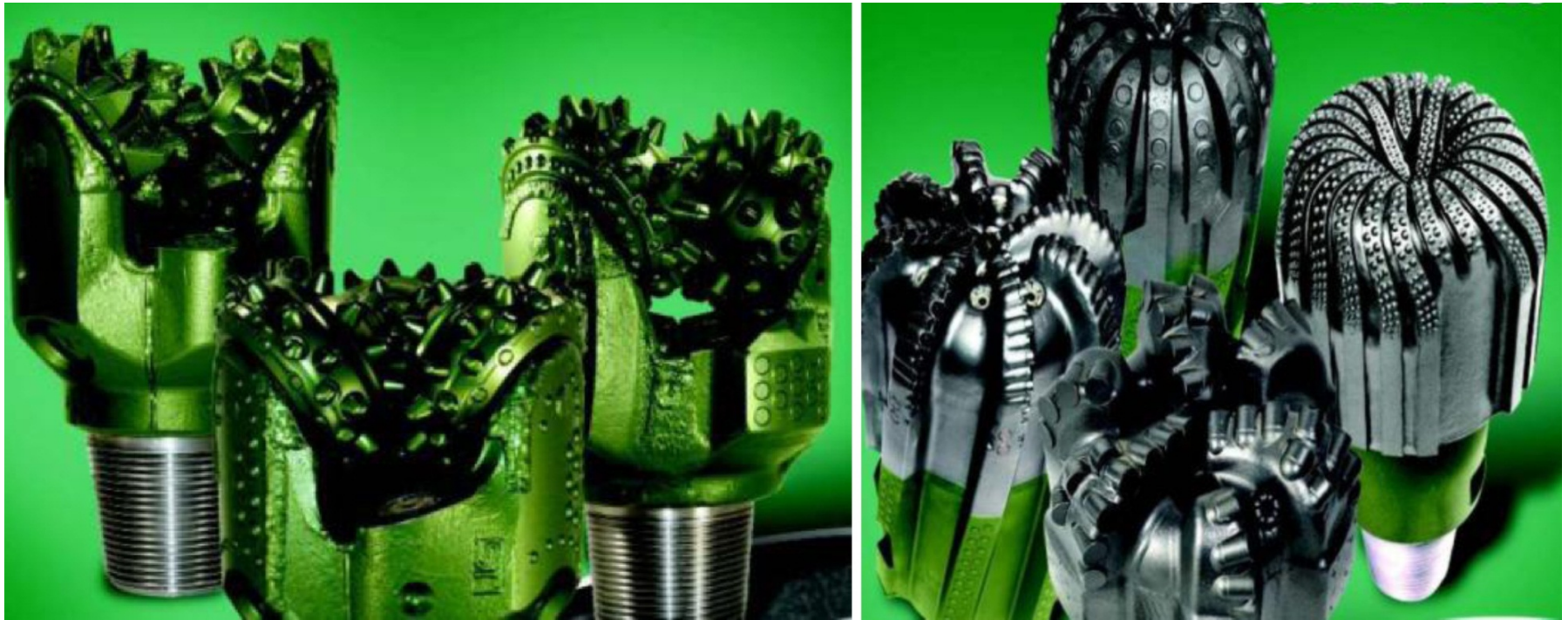
Figure 3.2: Tri-cone roller bits (left) and polycrystalline diamond compact (PDC) bits (right) (Ngugi, 2008).
