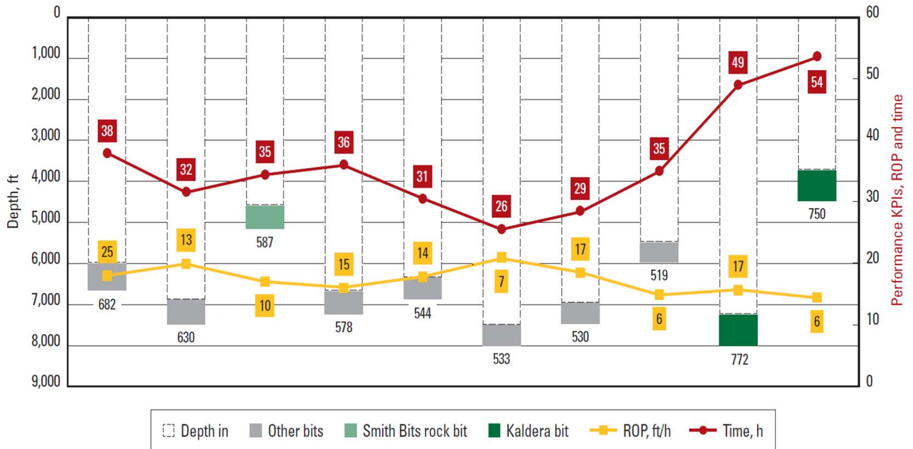
Figure 9.2: Kaldera drilling results at The Geysers: The Kaldera bit drilled 14 hours longer and approximately 150 feet farther than other bits, representing a run length increase of 25% (Schlumberger, 2013).
