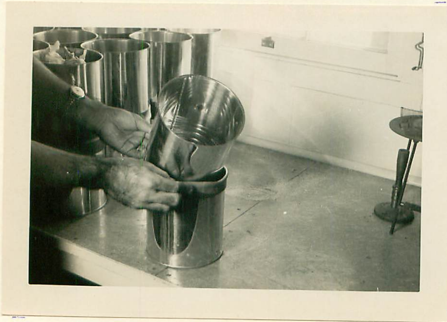
Figure 3.—Attaching cans by means of rubber tubing.
