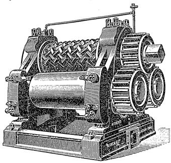
proved beyond doubt that the "Diamond" Roller not only increases the extraction of the mill, but that it does so with about two-thirds of the power required with ordinary rollers.
