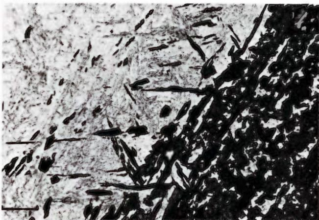
**Figure 1883.** Wallapai. Detail of the same field as Figure 1882. Transition from lightly etched to heavily etched (in reality brown, blue and black colors) martensite plates. Etched. Scale bar 20  $\mu$ . See also Figure 128.
