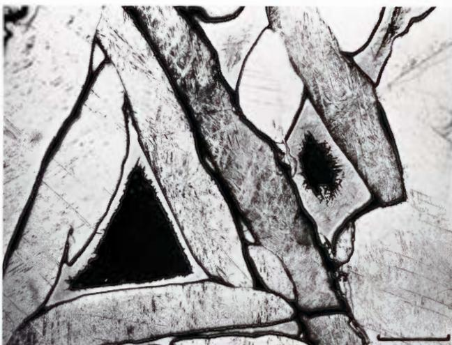
**Figure 1881.** Wallapai (Tempe no. 58bx). Shock-hatched kamacite and dark-etching plessite fields with cloudy taenite rims. Etched. Scale bar 400  $\mu$ .
