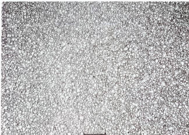
**Figure 1889.** Washington County (Harvard no. 565). Recrystallized even-sized kamacite grains with minute precipitates. Etched. Scale bar 500  $\mu$ .
