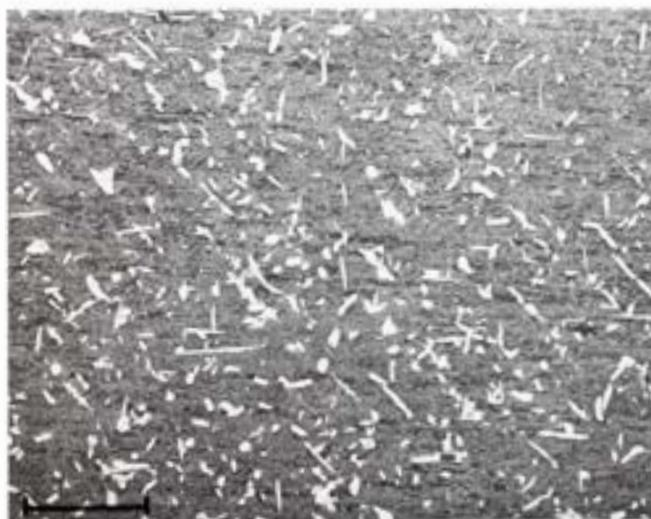
Figure 1907. Weaver Mountains (U.S.N.M. no. 1427). A nickel-rich ataxite of group IVB. Many of the kamacite spindles contain tiny nuclei of schreibersite. Etched. Scale bar 200  $\mu$ . (Perry 1950: volume 7.)
