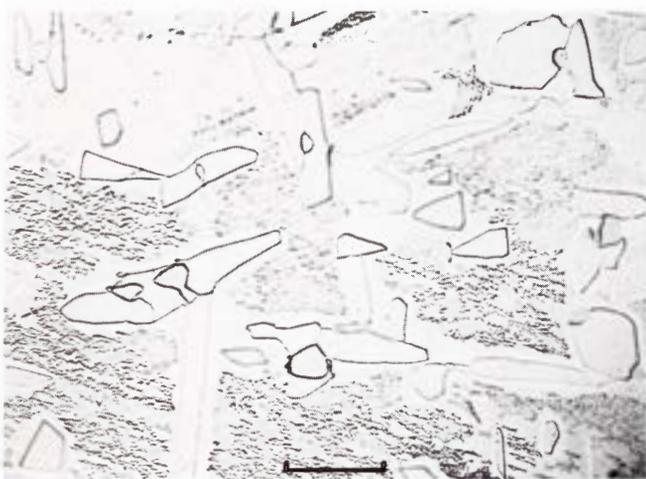
**Figure 1885.** Warburton Range (Los Angeles). A nickel-rich ataxite of group IVB. Kamacite spindles in an unresolvable duplex matrix. Fine schreibersite crystals inside several of the kamacite grains. Etched. Scale bar 50  $\mu$ .
