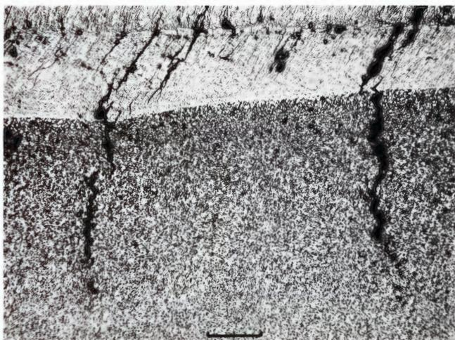
**Figure 1892.** Washington County. Detail of the fusion crust at F on Figure 1888 (inverted). The metallic fusion crust is composed of numerous layers of dendritic-columnar structure. Hot-cracks penetrate the crust and the heat-affected A zone (page 53). Compare Figure 51. Etched. Scale bar 500  $\mu$ .
