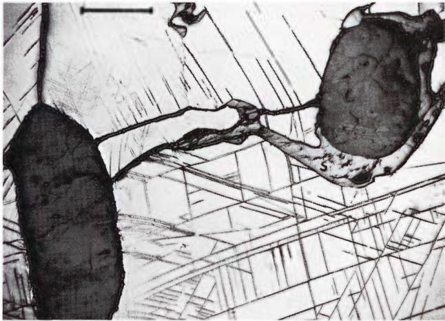
**Figure 1896.** Waterville (Tempe no. 453.2x). Two troilite nodules, the one at right having served as a substrate for precipitating schreibersite (S). Several differently oriented kamacite grains with Neumann bands. Compare Figure 163. Etched. Scale bar 400  $\mu$ .
