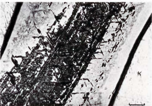
**Figure 1882.** Wallapai (Tempe no. 58bx). Plessite field between two kamacite lamellae (K). The plessite shows cloudy taenite edges and martensitic interiors, with plates developed parallel to the bulk Widmanstätten pattern. Etched. Scale bar 50  $\mu$ .
