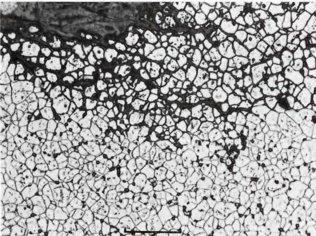
**Figure 1905.** Wathena (U.S.N.M. no. 1387). Near-surface section showing intergranular corrosion. The numerous black angular dots are sensitized loops that were preferentially attacked. Compare, e.g., Kopjes Vlei. Etched. Scale bar 200  $\mu$ .
