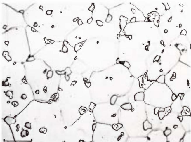
**Figure 1891.** Washington County (Harvard no. 565). A detail showing the irregular cavernous taenite particles and the angular, slightly darker phosphide particles. They are mainly located at grain boundaries, probably because these were pinned by the precipitates. Etched. Scale bar 40  $\mu$ .
