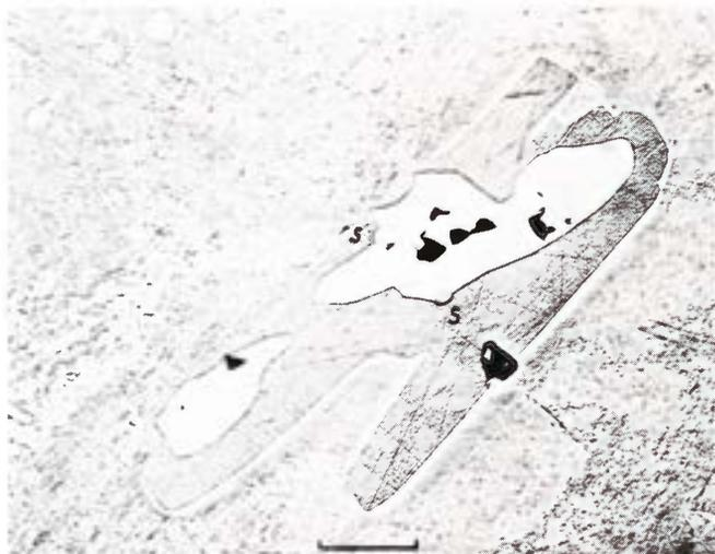
**Figure 1886.** Warburton Range (Los Angeles). Two schreibersite crystals (white, with chipped portions) inside kamacite spindles. Two small sulfide particles (S) are associated with the larger schreibersite crystal. Etched. Scale bar  $50 \mu$ .
