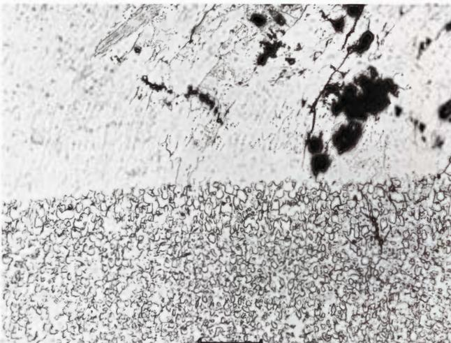
**Figure 1893.** Washington County (Harvard no. 565). The fusion crust (above) shows cellular-columnar growth with the crystals slightly tilted relative to the substrate. (Black denotes terrestrial corrosion products). The heat-affected  $\alpha_2$  zone is of a peculiar nature because it formed from a fine three-component mixture of  $\alpha$ ,  $\gamma$  and phosphides. Etched. Scale bar 200  $\mu$ .
