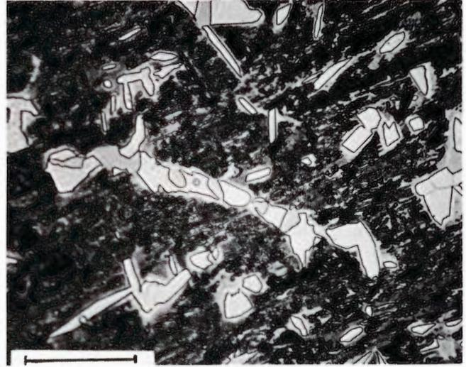
**Figure 1909.** Weaver Mountains (U.S.N.M. no. 1427). Kamacite grains with numerous schreibersite particles, usually in contact with taenite along at least one surface. Etched. Scale bar 40  $\mu$ . (Perry 1950: volume 7.)
