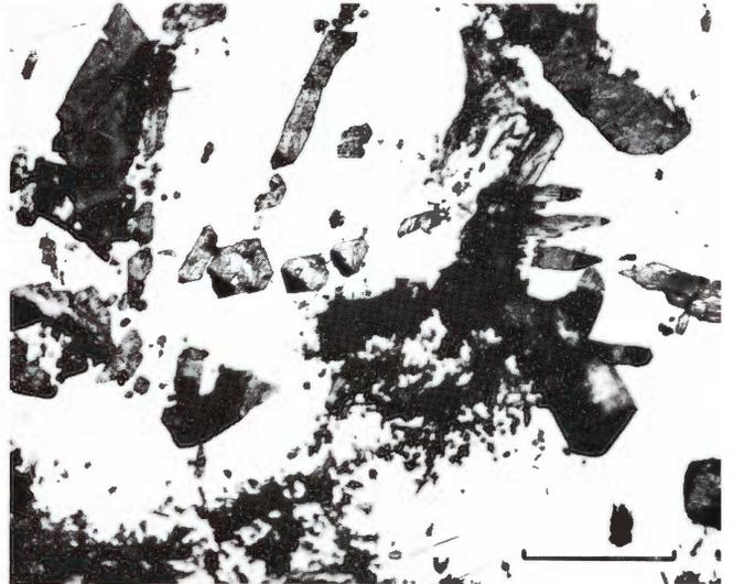
**Figure 1898.** Waterville (Tempe no. 453.2x). Kamacite (white) with a cluster of graphite particles typical for Waterville. Acicular and flaky particles occur besides irregular ones and some with cubic morphology. Polished. Crossed polars. Scale bar 100  $\mu$ .
