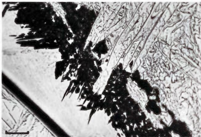
**Figure 1884.** Wallapai (Tempe no. 58bx). The edge of an acicular plessite field. Kamacite (K) is followed by a narrow yellow high nickel taenite edge. Then follows cloudy taenite and martensitic transition zones. The interior is shock-hatched kamacite needles between taenite lamellae. Etched. Scale bar 20  $\mu$ .
