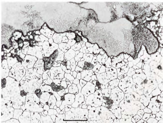
**Figure 1902.** Wathena (U.S.N.M. no. 1387). The edge of a shock-melted troilite nodule. Small sulfide blebs have in the process become detached and are now situated outside the serrated boundary. Recrystallized kamacite with minute phosphide particles. Etched. Scale bar 200  $\mu$ .
