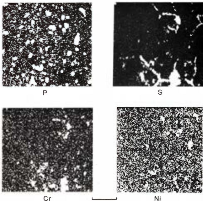
**Figure 1903.** Wathena (U.S.N.M. no. 1387). X-ray scanning pictures of shock-melted sulfide filaments outside a nodule similar to Figure 1902. The filaments are basically remelted troilite and daubreelite material, while phosphides occur as discrete particles.  $PK_{\alpha}$ ,  $SK_{\alpha}$ ,  $CrK_{\alpha}$ , and  $NiK_{\alpha}$  pictures at 15KV. Scale bar 50  $\mu$ . See also Figure 178.
