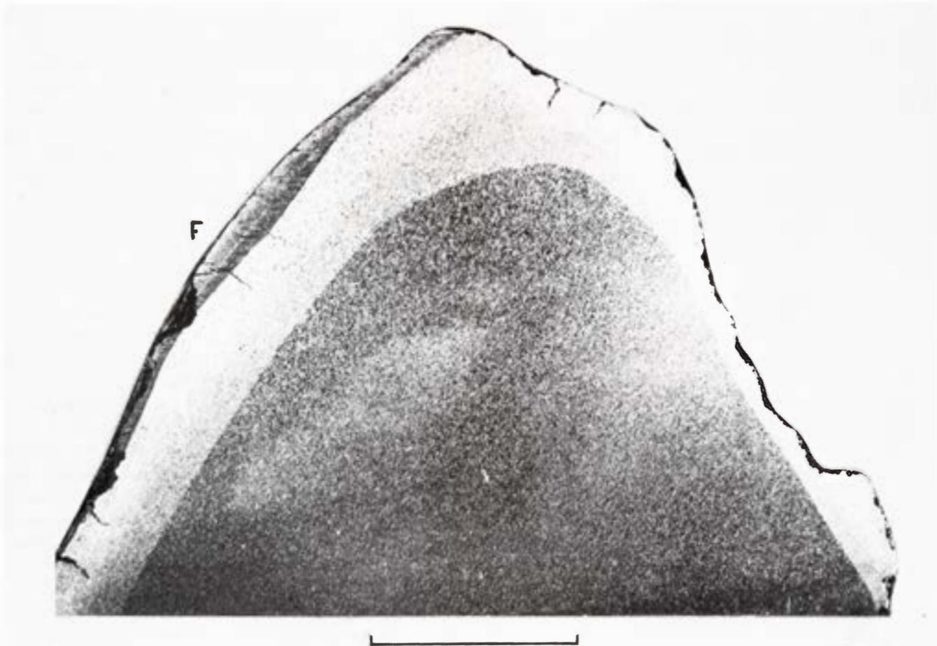
Figure 1888. Washington County (Harvard no. 565). A section taken where the flat regmaglypt-covered side (right) meets the smooth domed side (left). The width of the heat-affected  $\alpha_2$  zone is 3-4 times larger under the domed side, which is also covered with layered fusion crusts. Evidently the ablation rate was highest on the regmaglypt-covered side. Etched. Scale bar 10 mm.
