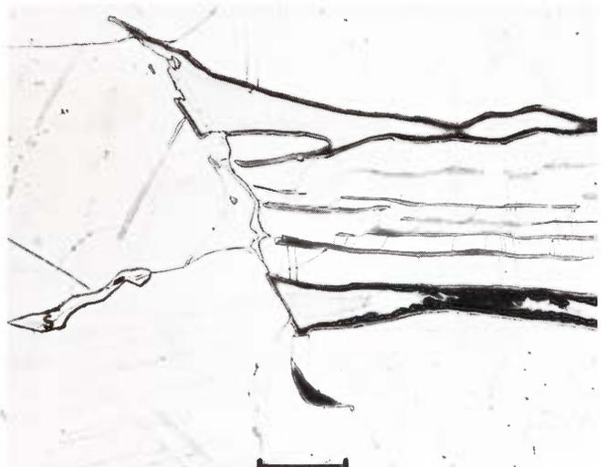
**Figure 1899.** Waterville (Tempe no. 453.2x). A comb plessite field and a schreibersite crystal (S) in a grain boundary. The plessite shows cloudy taenite edges and martensitic interiors. Etched. Scale bar 200  $\mu$ .
