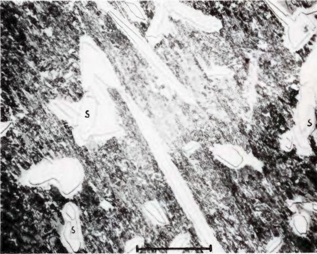
**Figure 1908.** Weaver Mountains (U.S.N.M. no. 1427). Kamacite grains with schreibersite crystals (S). Duplex, almost unresolvable matrix. Etched. Scale bar 50  $\mu$ . (Perry 1950: volume 7.)
