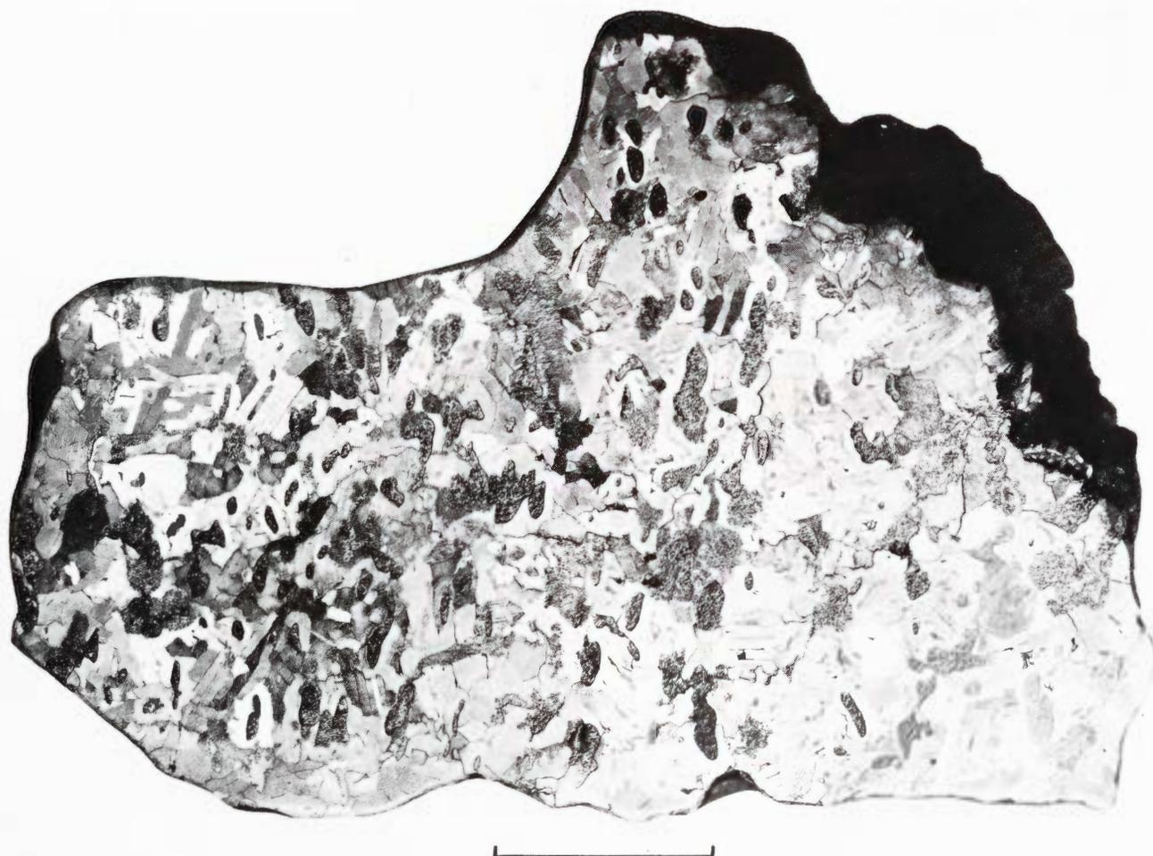
Figure 1895. Waterville (U.S.N.M. no. 1512; 149 g). An anomalous polycrystalline aggregate with abundant troilite and graphite. Deep-etched. Scale bar 20 mm. S.I. neg. 41117A.
