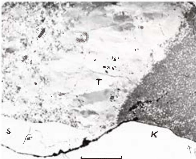
**Figure 1897.** Waterville (Tempe no. 453.2x). Troilite (T), schreibersite (S) and kamacite (K) with an unidentified component to the right. The troilite shows recrystallized portions (left) and portions with undulatory extinction (center). Polished. Crossed polars. Scale bar 100  $\mu$ .
