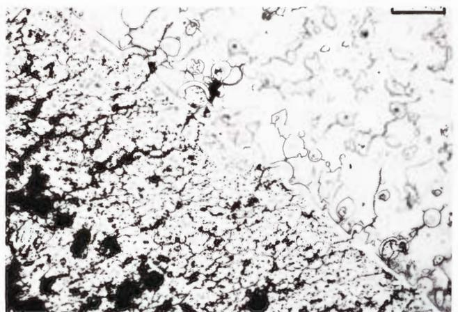
**Figure 1894.** Washington County (Harvard no. 565). Fusion crust (left) with terrestrial corrosion products at cell boundaries (black). The heat-affected  $\alpha_2$  zone shows globular phosphide melts with gas holes. Etched. Scale bar 50  $\mu$ .
