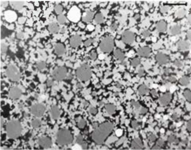
**Figure 1904.** Wathena (U.S.N.M. no. 1387). Detail of the massive shock-melted troilite. In a fine-grained eutectic of iron (black) and sulfide (gray) nearly molten particles of daubreelite (dark gray) and schreibersite (white) are dispersed. Etched (thereby the iron component was removed, leaving black grooves). Oil immersion. Scale bar 10  $\mu$ .
