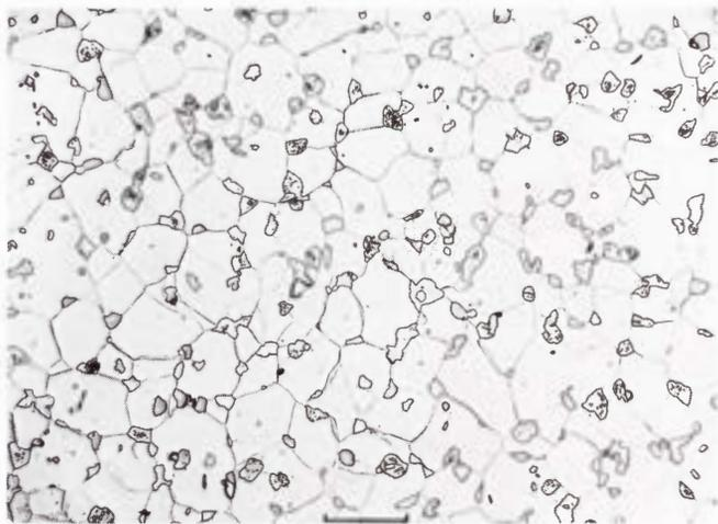
**Figure 1890.** Washington County (Harvard no. 565). Polycrystalline kamacite with amoebae-shaped taenite particles and angular phosphide particles. No Neumann bands. Etched. Scale bar 50  $\mu$ .
