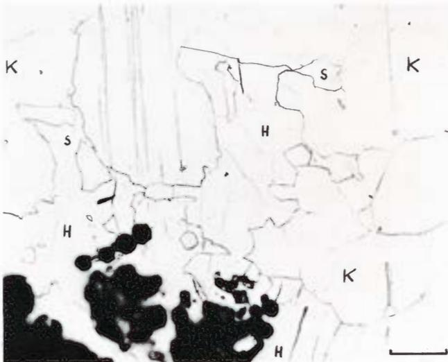
**Figure 1877.** Walker County (U.S.N.M. no. 379). Detail of the edge of another graphite nest similar to that in Figure 1876. A cluster of fine cliftonitic graphite crystals (black) are located in kamacite (K) with Neumann bands, and in haxonite (H) with small phosphide inclusion (S). Etched. Scale bar  $50 \mu$ .
