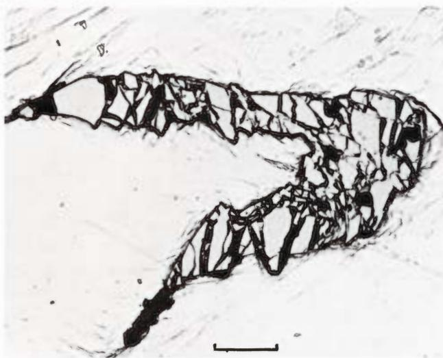
**Figure 2086.** Imilac (Copenhagen). A schreibersite crystal which has been entirely brecciated during the deformation. Etched. Scale bar 25 μ.
