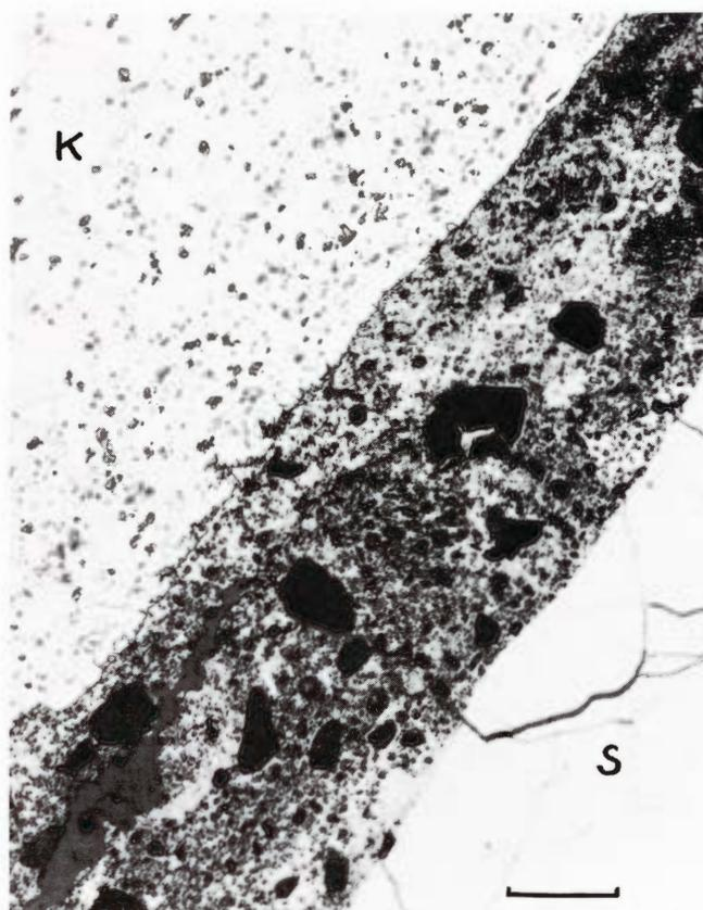
**Figure 2087.** Imilac (Copenhagen). A shear zone through a 15 g fragment. A mobile troilite melt has been injected along the fissured interface between schreibersite (S) and kamacite (K). In the troilite are numerous olivine fragments (black). Etched. Scale bar 25 μ.
