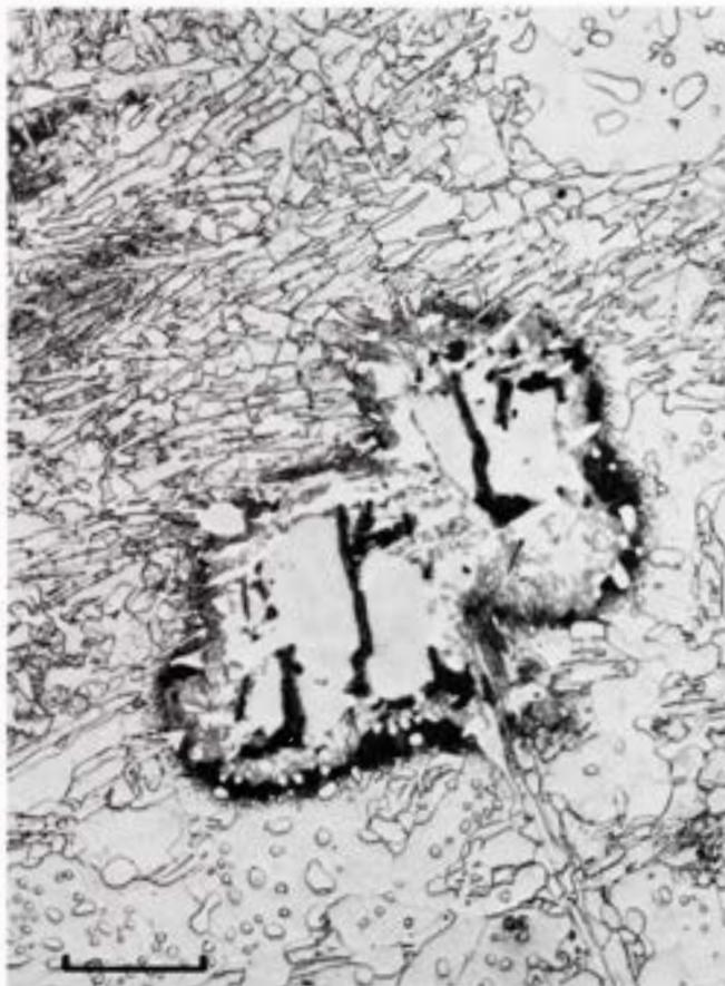
**Figure 2101.** Magnesia. A carbide 'rose' which happened to be located in the heat-affected  $\alpha_2$  zone and started to decompose. Carbon that diffused away from the haxonite formed a supersaturated austenite that, upon cooling, transformed to martensitic and bainitic structures according to the local nickel and carbon level. Some graphitization also occurred. Etched. Scale bar  $50\ \mu$ .
