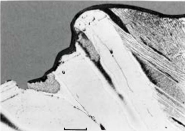
**Figure 2094.** Magnesia (Paris). A polished and etched section that includes the late fracture surface. The linear structural elements are distorted and the surface is partially covered by a thin laminated fusion crust. Scale bar 0.5 mm.
