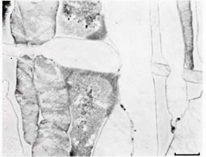
**Figure 2095.** Magnesia. Typical view of alternating shock-hatched kamacite and taenite and plessite fields. The whitish blebs inside some plessite fields are the carbide 'roses', composed of haxonite, taenite, kamacite and schreibersite. Etched. Scale bar 0.5 mm.
