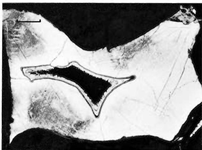
Figure 2081 B. Imilac (Copenhagen). The metallic parts of a pallasite form an almost continuous sponge with olivine crystals (black) in the interstices. The metal of the photograph was at high temperature a single taenite crystal; on cooling, kamacite was nucleated on the olivine crystals and grew toward the center. This became enriched in nickel (and carbon) and finally decomposed to bainitic-martensitic transformation products. Etched. Scale bar 400  $\mu$ .
