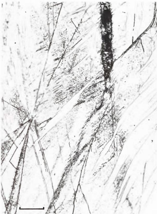
**Figure 2084.** Imilac (Copenhagen). Distorted kamacite with lenticular deformation bands and precipitates of submicron size. Etched. Scale bar 100  $\mu$ .
