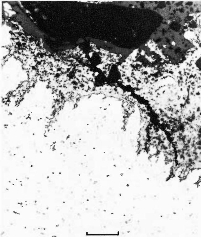
**Figure 2088.** Imilac (Copenhagen). The edge of a fused troilite pool with an olivine fragment (black). The troilite penetrates in an irregular way into the thermally altered kamacite. Corrosion products are dark gray. Etched. Scale bar 25  $\mu$ .
