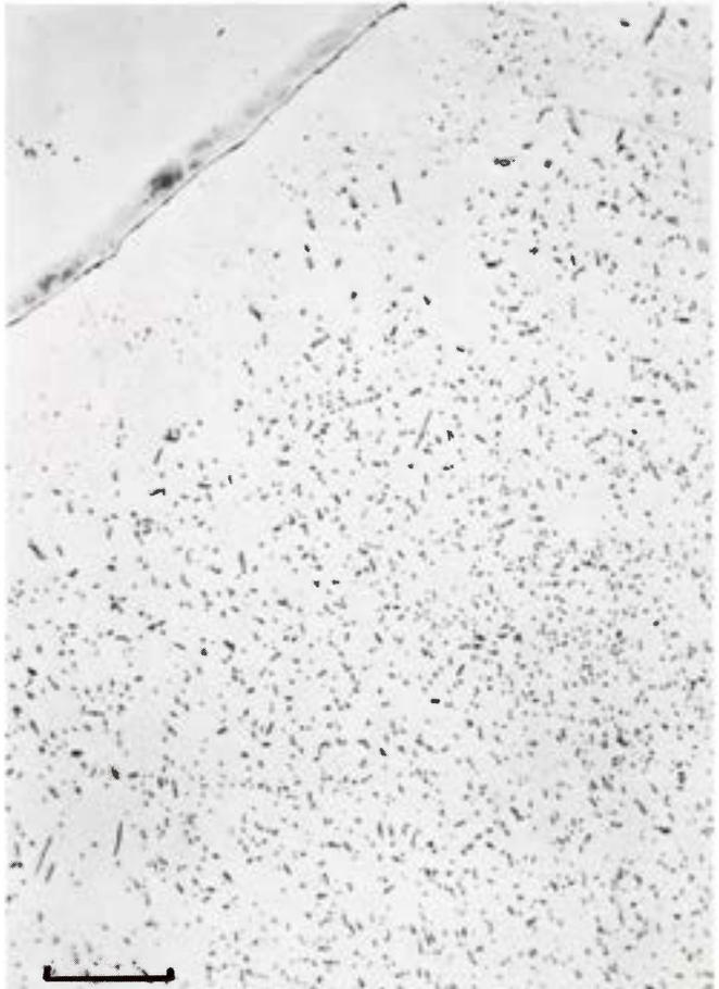
**Figure 2099.** Magnesia. In the kamacite are numerous densely spaced, micron-sized rhabdite particles. Above left, a cloudy taenite rim. Etched. Scale bar  $50 \mu$ .
