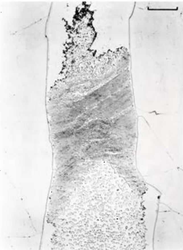
**Figure 2097.** Magnesia. A wide taenite ribbon which is under decomposition to spheroidized (below) and pearlitic plessite (center). Subboundaries in the kamacite lamellae on either side. Etched. Scale bar  $50 \mu$ .
