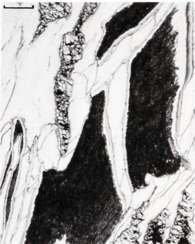
**Figure 2083.** Imilac (Copenhagen). Distorted metallic matrix caused by violent fragmentation. Several schreibersite crystals have been sheared and fragmented while the kamacite yielded plastically. Etched. Scale bar 100  $\mu$ .
