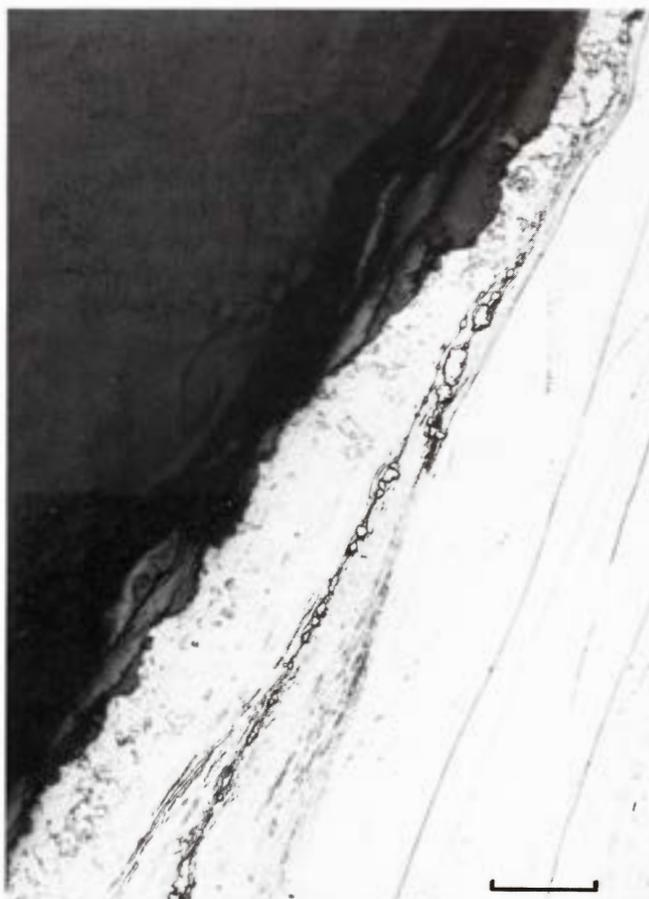
**Figure 2085.** Imilac (Copenhagen). The surface of a typical fragment produced by violent shear forces. A 100 μ wide zone adjacent to the shear fracture has been momentarily reheated so much, that the cold-worked kamacite recrystallized to imperfect 5-10 μ units. A schreibersite crystal has been torn asunder, and the fragments have become aligned along the shear zone. Etched. Scale bar 100 μ.
