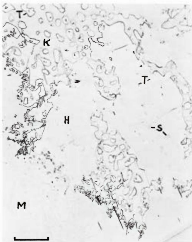
**Figure 2100.** Magnesia. An enlarged view of a carbide 'rose' like those of Figure 2095. Pure taenite (T) and schreibersite (S) particles are embedded in haxonite (H), which evidently is a rather late precipitate. Martensitic plessite (M) and kamacite is also apparent. Etched. Scale bar  $40\ \mu$ .
