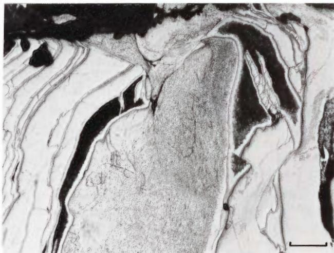
**Figure 2082.** Imilac (Copenhagen). Section through a 20 g distorted fragment. Severe shear zones penetrate the material and the structural elements are twisted or offset. Etched. Scale bar 400  $\mu$ .
