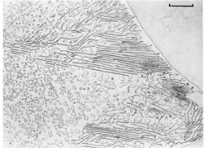
**Figure 2098.** Magnesia. Another example upon taenite under decomposition to mixed spheroidized and lamellar textures. Etched. Scale bar  $50 \mu$ .
