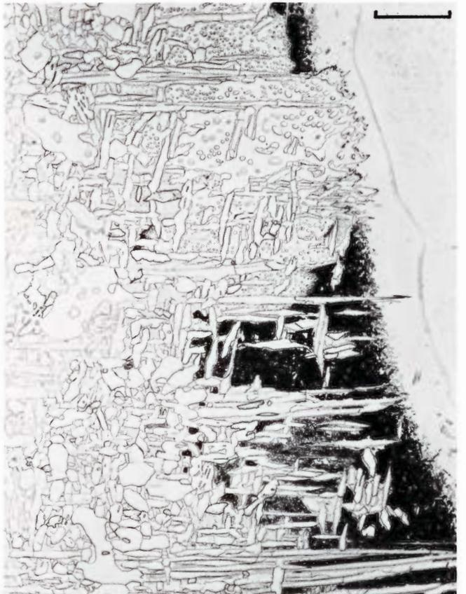
**Figure 2096.** Magnesia. A plessite field with acicular kamacite, spheroidized taenite particles and unresolvable black taenite. A narrow rim of cloudy taenite adjacent to kamacite, above right. Etched. Scale bar 50  $\mu$ .
