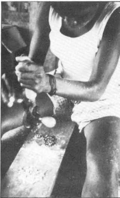
A woman uses modern drilling methods with a brace and bit; drilled pieces are in the foreground.
