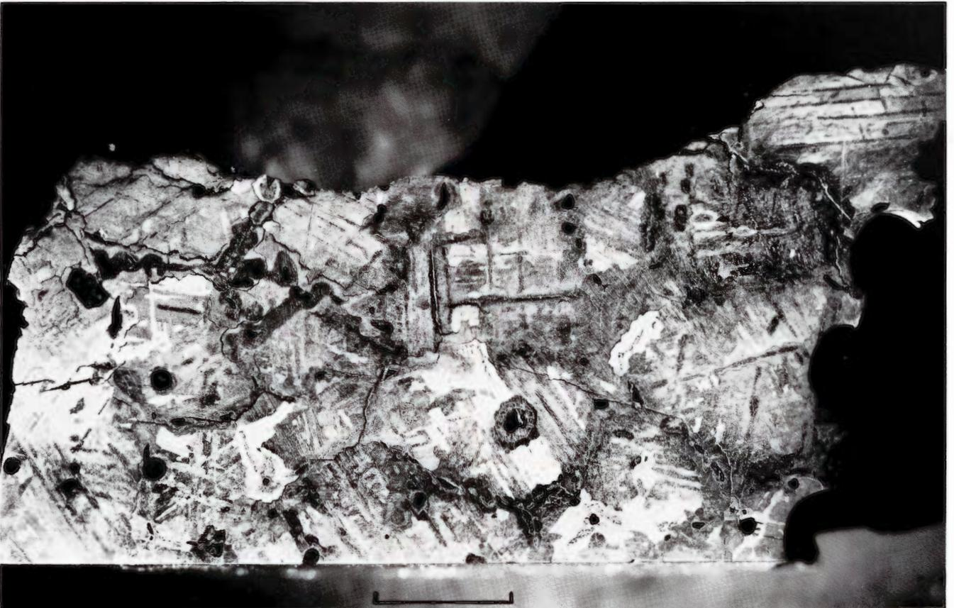
**Figure 2032.** Zacatecas (1792). (Brit. Mus. no. 28296; 2,570 g). A fine picture that shows the polycrystallinity, with troilite filaments at grain boundaries and troilite globules in the grain interiors. To the right, part of the drill holes shown in Figure 2026. Deep-etched. Scale bar 2 cm. B.M. neg. 5576.
