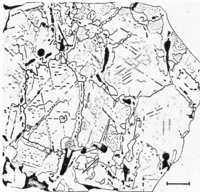
**Figure 2028.** Zacatecas (1792). An instructive drawing by Rose (1864a) that shows the polycrystalline nature and the numerous streaks of rhabdite crystals. Black nodules are troilite. Scale bar 10 mm.
