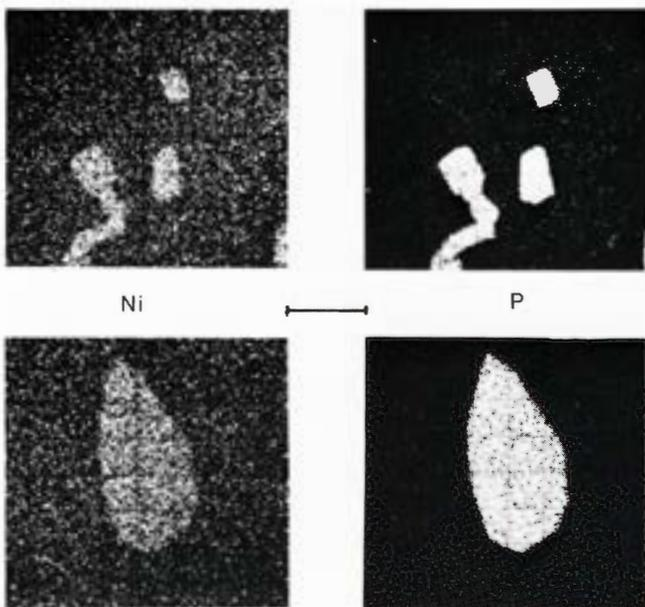
**Figure 2037.** Zacatecas (1792) (Copenhagen no. 1906, 145), X-ray scanning pictures of various inclusions, large and small, confirmed that they were essentially phosphides with relatively low (<15%) nickel contents. This, and their peculiar morphology, is probably the result of cosmic annealing. NiK<sub>α</sub> and PK<sub>α</sub> pictures at 15KV. Scale bar 100 μ.
