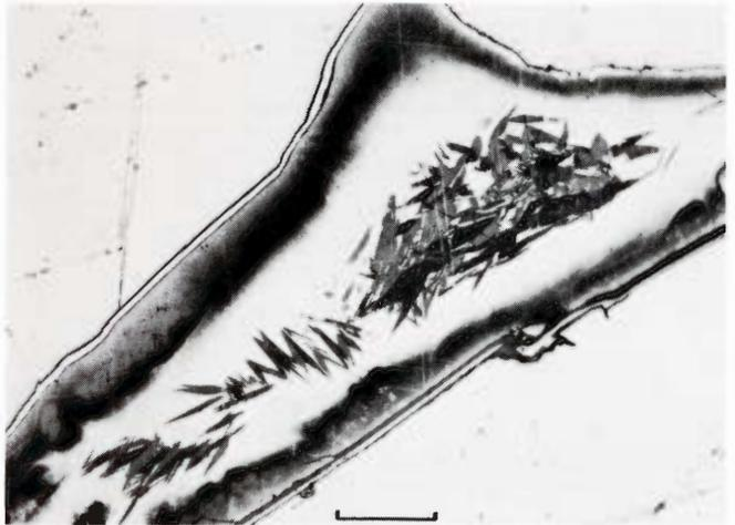
**Figure 2043.** Zaffra (Brit. Mus. no. 1963, 529). Taenite field with a high nickel content, presumably above 30% everywhere. The interior shows acicular carbon-nickel martensite. Terrestrial corrosion has selectively attacked along the interface with kamacite and along the inner edge of the  $2\text{-}3 \mu\text{m}$  wide yellow high-nickel taenite rim, so that this has become detached as a narrow uncorroded strip. Etched. Scale bar  $40 \mu\text{m}$ .
