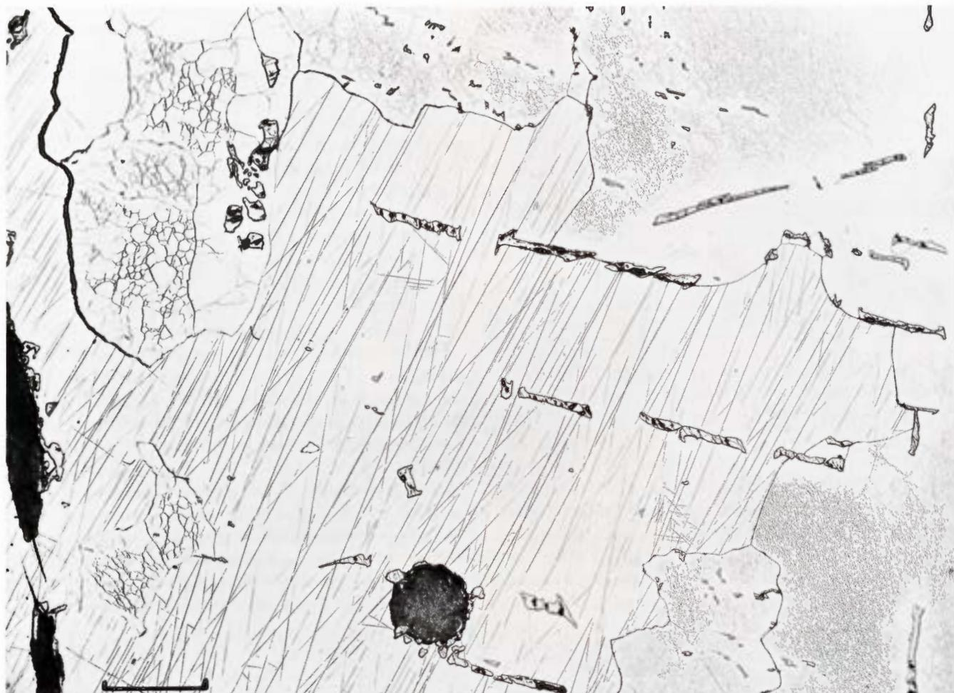
**Figure 2029.** Zacatecas (1792) (Copenhagen no. 1906, 145). Grain growth on part of the kamacite. To the left two areas with polygonization which resist recrystallization. Shock-melted troilite (black) with shattered schreibersite rims. Prominent rhabdites and Neumann bands. Etched. Scale bar 2 mm.
