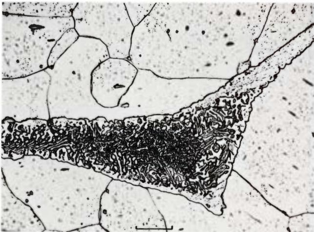
Figure 2047. Zerhamra (Copenhagen no. 1972, 1680). An annealed and decomposed plessite field. The interior is pearlitic or spheroidized, while the nickel-rich edge shows a dense  $(111)_\gamma$  grid with fine  $\alpha$ -precipitates. Etched. Scale bar  $50\ \mu$ .
