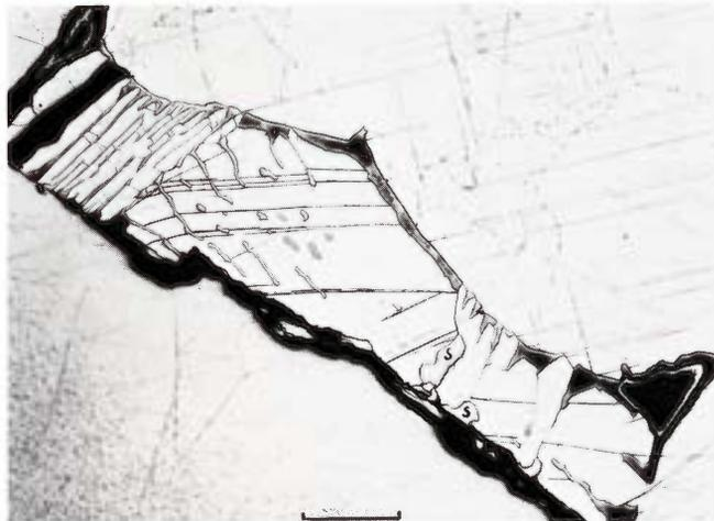
**Figure 2041.** Zaffra (Brit. Mus. 1963, 529). Open-meshed degenerated plessite field with schreibersite inclusions (S). Terrestrial limonite along lower interface. Neumann bands in the kamacite. Etched. Scale bar 400  $\mu$ .
