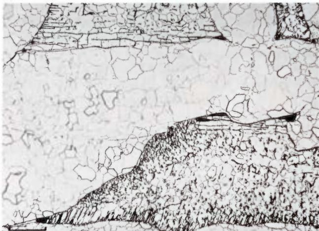
**Figure 2045.** Zerhamra (Copenhagen no. 1972, 1680). A recrystallized medium octahedrite, probably belonging to group IIIA. The equiaxial kamacite grains are slightly smaller within the degenerated plessite fields than within the kamacite lamellae. Etched. Scale bar 500  $\mu$ .
