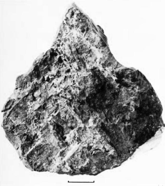
**Figure 2039.** Zacatecas (1969). The same from the opposite side showing that the base is a hackly fracture surface with distinct parting along schreibersite-rich Widmanstätten boundaries. Scale bar 3 cm. S.I. neg. 1606C.
