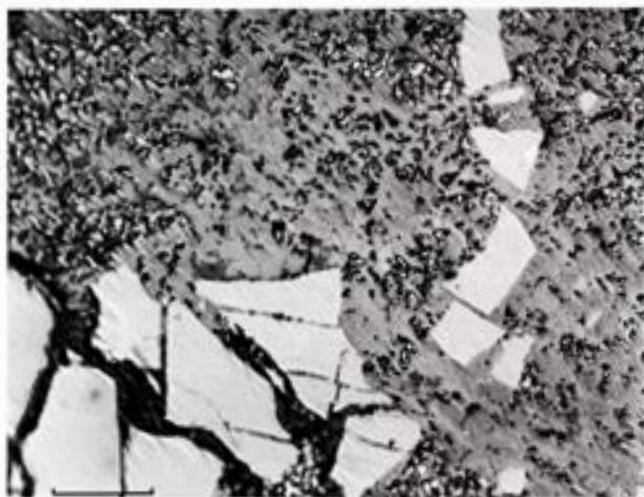
**Figure 2035.** Zacatecas (1792) (Copenhagen no. 1906, 145). Shock-melted polycrystalline troilite in which are embedded angular fragments of schreibersite, previously located along the troilite-kamacite interface. Etched. Scale bar 20  $\mu$ .
