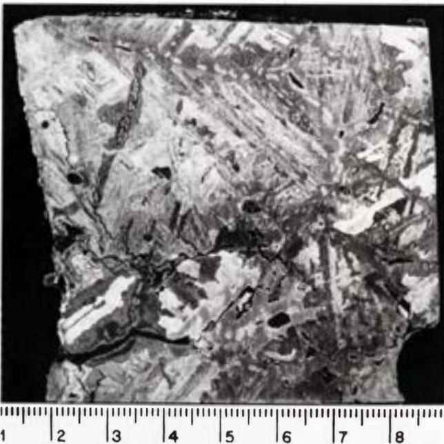
**Figure 2027.** Zacatecas (1792) (Tempe no. 232.1). Inch-sized precursor taenite grains have each transformed to an indistinct Widmanstätten pattern. In the grain boundaries are troilite and schreibersite inclusions. Deep-etched. Scale in centimeters. (Courtesy C.B. Moore.)
