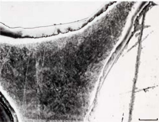
**Figure 2042.** Zaffra (Brit. Mus. no. 1963, 529). Martensitic plessite field with cloudy taenite edges. Terrestrial corrosion has attacked the duplex interior and the cloudy rim zone. The decorated Neumann bands (right) are also selectively attacked. Etched. Scale bar  $50 \mu\text{m}$ .
