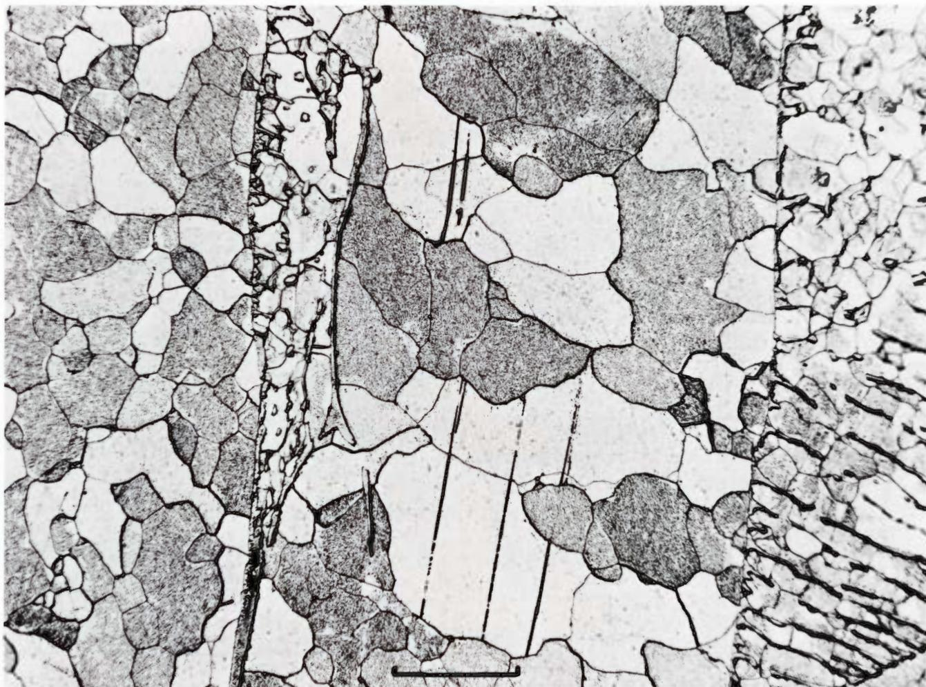
**Figure 2046.** Zerhamra (Copenhagen no. 1972, 1680). Near some of the surface cracks a few of the recrystallized kamacite grains contain a new generation of Neumann bands, probably dating from the atmospheric deceleration. Etched. Scale bar 300  $\mu$ . See also Figure 100.
