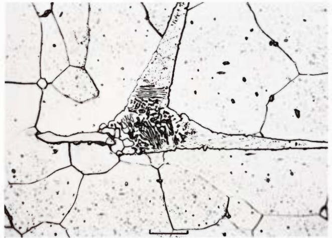
Figure 2048. Zerhamra (Copenhagen no. 1972, 1680). Another annealed plessite field and a schreibersite crystal (S) with fine  $\gamma$ -particles along its periphery. Etched. Scale bar  $50\ \mu$ .
