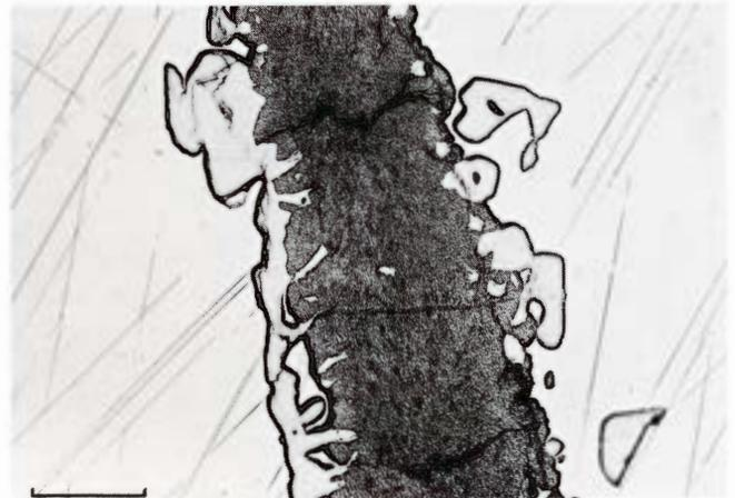
**Figure 2034.** Zacatecas (1792). Detail of left edge of Figure 2029. Shock-melted troilite (gray) and brecciated schreibersite bodies, apparently healed by a subsequent annealing period. Etched. Scale bar 300  $\mu$ .
