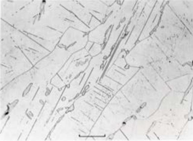
**Figure 2031.** Zacatecas (1792). (Copenhagen no. 1906, 145). An area with elongated kamacite grains. Schreibersite (or rhabdite) particles are common, while taenite is absent. Etched. Scale bar 300  $\mu$ . See also Figure 173.
