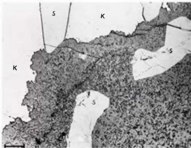
**Figure 2036.** Zacatecas (1792) (Brit. Mus. no. 33917). Another sample of shock-melted troilite with dispersed schreibersite fragments (S). Serrated, unequilibrated interface with kamacite (K). Etched. Scale bar 50  $\mu$ .
