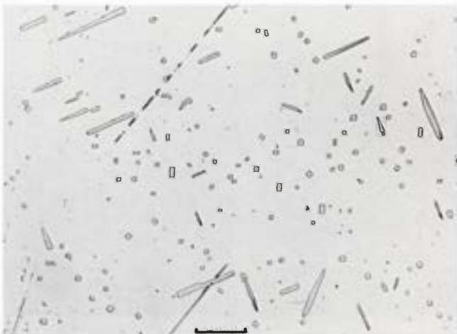
**Figure 2033.** Zacatecas (1792). (Copenhagen no. 1906, 145). A kamacite crystal with prismatic rhabdites. An annealed Neumann band above left. Etched. Scale bar 100  $\mu$ .
