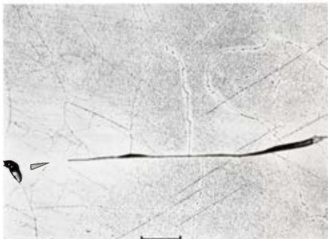
**Figure 2040.** Zaffra (Brit. Mus. no. 1963, 529). Cloudy taenite lamella with grain boundary schreibersite at either end. Kamacite with subboundaries that are pinned by phosphide particles. Etched. Scale bar 500  $\mu$ .
