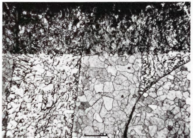
Figure 2049. Zerhamra (Copenhagen no. 1972, 1680). Heat-affected  $\alpha_2$  zone (above) and unaffected interior. It is quite clear that the kamacite is annealed and without Neumann bands. Etched. Scale bar  $500\ \mu$ .
