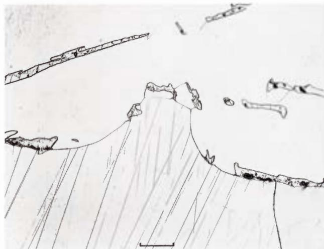
**Figure 2030.** Zacatecas (1792). Detail of Figure 2029 showing a moving grain boundary that was pinned by rhabdite crystals. Neumann bands are present in both grains, but due to orientation not so sensitive to the etching reagent (Nital) in the upper grain. Etched. Scale bar 500  $\mu$ .
