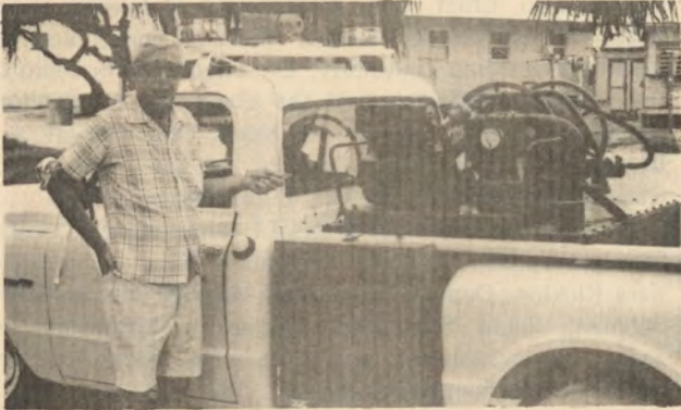
Ebeye Public Works Director Fred Hanson stands next to his newest acquisition, the island's only piece of mobile fire-fighting equipment. It is a pickup truck-mounted pump, and should assist in fighting the frequent house fires on the congested island. Hanson also hopes to obtain a fire engine through Kwajalein sources.
