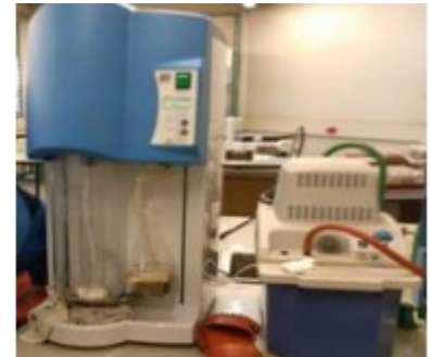
Figure 6: Distillation machine used to analyse 20 ml of supernatant collected (AMN analysis).
