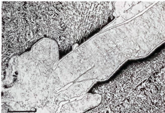
Figure 620. Chupaderos (Tempe no. 31a). Such \alpha_2 transformation is common in near-surface heat-affected samples. Etched. Scale bar 400 \mu .
