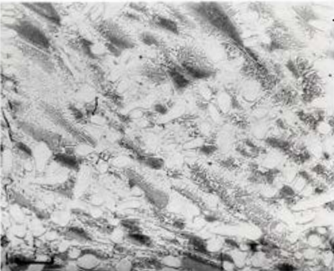
Figure 623. Chupaderos (Tempe no. 31a). Fused and rapidly solidified schreibersite lamella, which remained in its rounded cavity. Another part was lost as finely disseminated droplets during atmospheric ablation. Lightly etched. Scale bar 50\ \mu .
