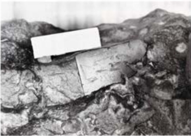
Figure 614. Chupaderos. Detail of Figure 613, upper left part. The rough, polished and etched section clearly shows the numerous schreibersite skeleton crystals. Ruler 15 cm.
