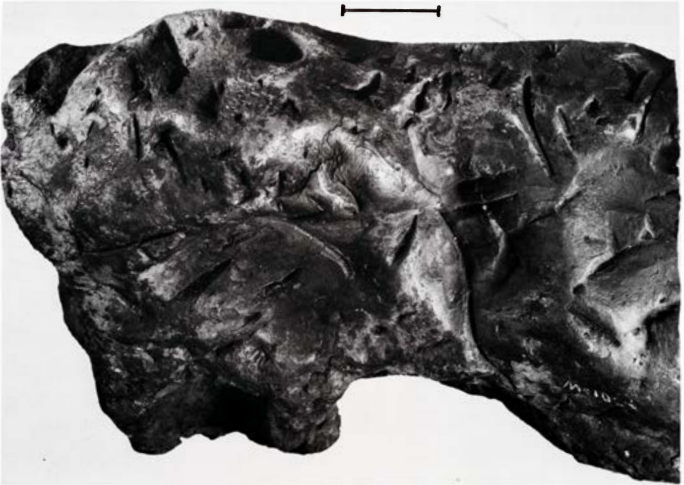
Figure 626. Chupaderos. Half of the Cuernavaca mass, now in Chicago (Chicago no. 1025, 17.3 kg). Eminent fusion crust and deep scars from ablated schreibersite lamellae. See also Figure 191. Scale bar 3 cm. S.I. neg. M-110A.
