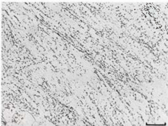
Figure 621. Chupaderos (Tempe no. 31a). The preatmospheric kamacite structure was apparently an annealed shock-hatched transformation product. Very fine beads of taenite and phosphides occur everywhere. Etched. Scale bar 20 \mu .
