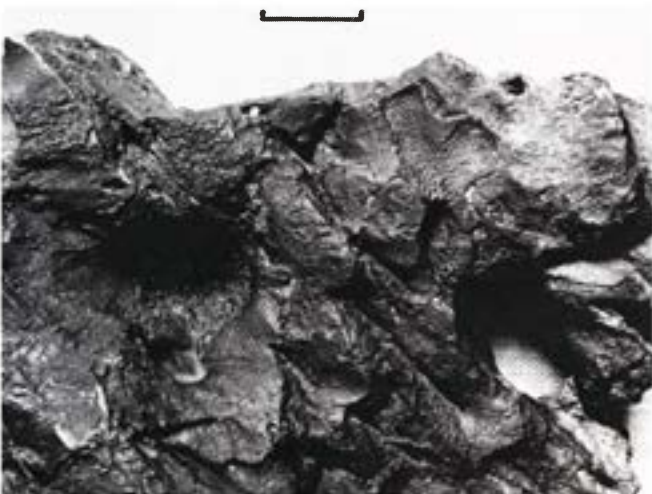
Figure 615. Chupaderos (Institute of Geology, Mexico City, no. 61). An endpiece which shows eminent orange peel fusion crust and chisel-like scars from ablated schreibersite plates. Scale bar 2 cm.
