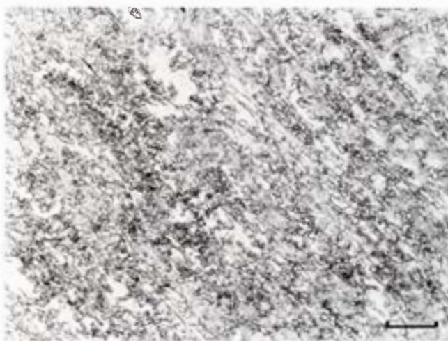
Figure 608. Chinga. Detail of Figure 605. The matrix appears to be an imperfectly annealed duplex \alpha + \gamma structure, with mostly submicroscopic particles. Etched. Oil immersion. Scale bar 10 \mu .
