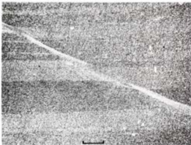
Figure 605. Chinga (U.S.N.M. no. 1426; cut from Moscow no. 537). Ataxitic structure at low magnification. A significant shear zone extends diagonally across the picture. See also Figure 207. Etched. Scale bar 500 \mu .
