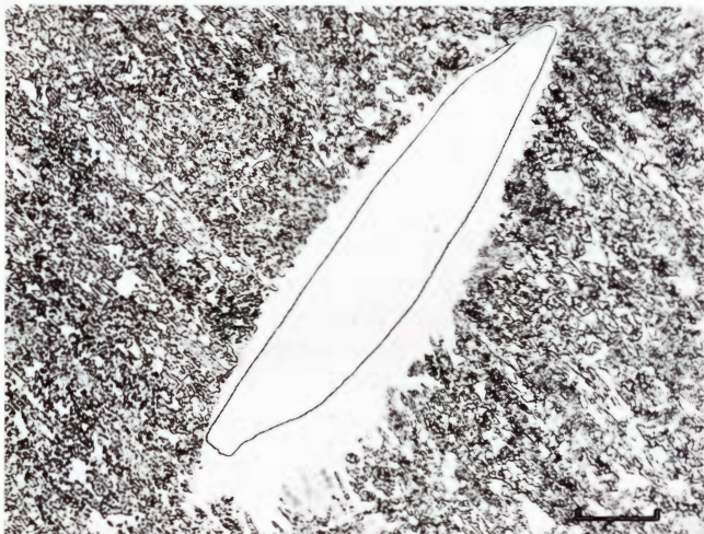
Figure 607. Chinga. Detail of Figure 605. A kamacite spindle with its enveloping undecomposed, high-nickel taenite rim. Etched. Oil immersion. Scale bar 10 \mu .
