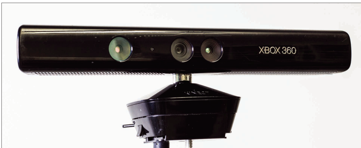
Figure 2. The Microsoft Kinect sensor for Xbox 360, or V1. The leftmost circular window is the IR emitter, the middle window is the RGB camera, and the rightmost window is the IR camera.
