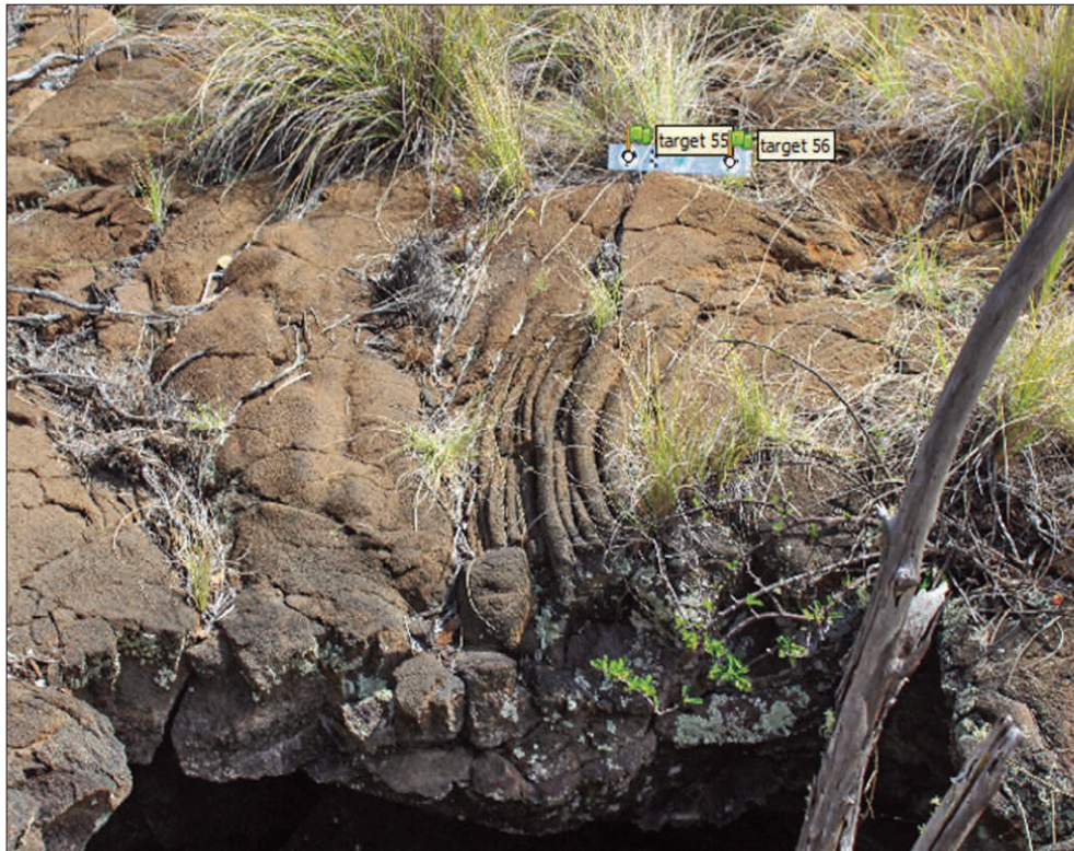
Figure 3. Agisoft PhotoScan image of a lava tube opening (at the bottom of the photograph) demonstrating the ability of the software to locate calibrated photogrammetric scale bars (with 12-bit coded targets) designed by personnel at the Bureau of Land Management’s National Operations Center for Photogrammetry, and sold by Cultural Heritage Imaging (CHI). Photographed by Paul White, UAA.
