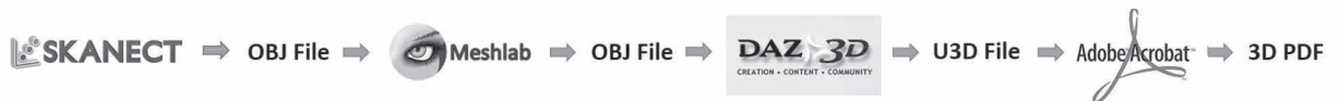
Figure 8. A workflow that allows the creation of 3D PDFs from virtually any 3D modeling program. Workflow and chart adapted from Porter (2015), and used with permission.
