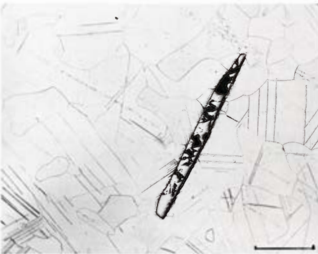
Figure 1777. Tombigbee (U.S.N.M. no. 252). Entirely recrystallized kamacite with a chipped schreibersite crystal. A late generation of Neumann bands penetrates all the recrystallized grains, probably dating from atmospheric breakup. Etched. Scale bar 200 \mu . (Perry 1944: plate 5.) See also Figure 221.
