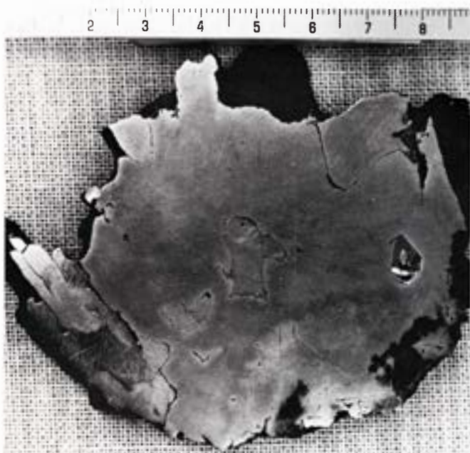
Figure 1776. Tombigbee (Tucson no. 825). An unusual sample showing remnant coarse Widmanstätten structure in the left side. Taenite and plessite are also indistinctly seen. To the right, a schreibersite skeleton crystal. Deep-etched. Scale in centimeters.
