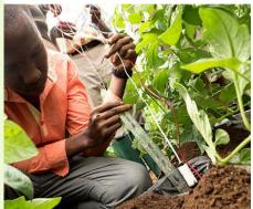
The Chameleon is a soil moisture tensor sensor that measures how much suction a plant must apply to get water out of the soil. With a simple 'traffic light' display unit that lights up in red, blue, or green, depending on the amount of moisture present, farmers can gauge if they are adequately irrigating their crops.
