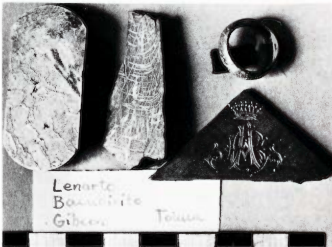
Figure 23. Examples of worked iron meteorites of known origin. A forged plate of Lenarto, a coldhammered wedge of Bacubirito, a forged finger ring of Gibeon, and a triangular slab of Toluca with the initials AB, probably those of Aristides Brezina. The specimens are now in the Vienna Museum. Scale bar in centimeters.
