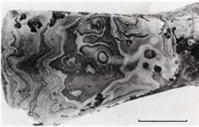
Figure 22. A medieval (?) adze blade (535 grams) exhibiting damascene pattern on the polished and etched surface. Microprobe examination indicates that the adze was produced by forging alternating layers of mild steel and meteoritic, probably hexahedritic, material. The adze was excavated in Central Sweden and is in private possession. Scale bar approximately 3 cm.
