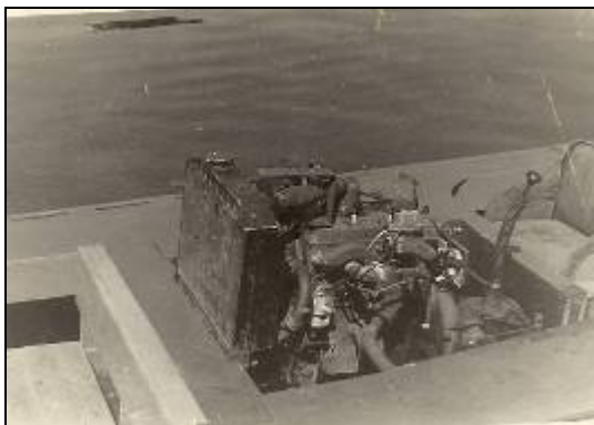
Boat powered by Jeep engine, Tombolo, Italy, 1946
