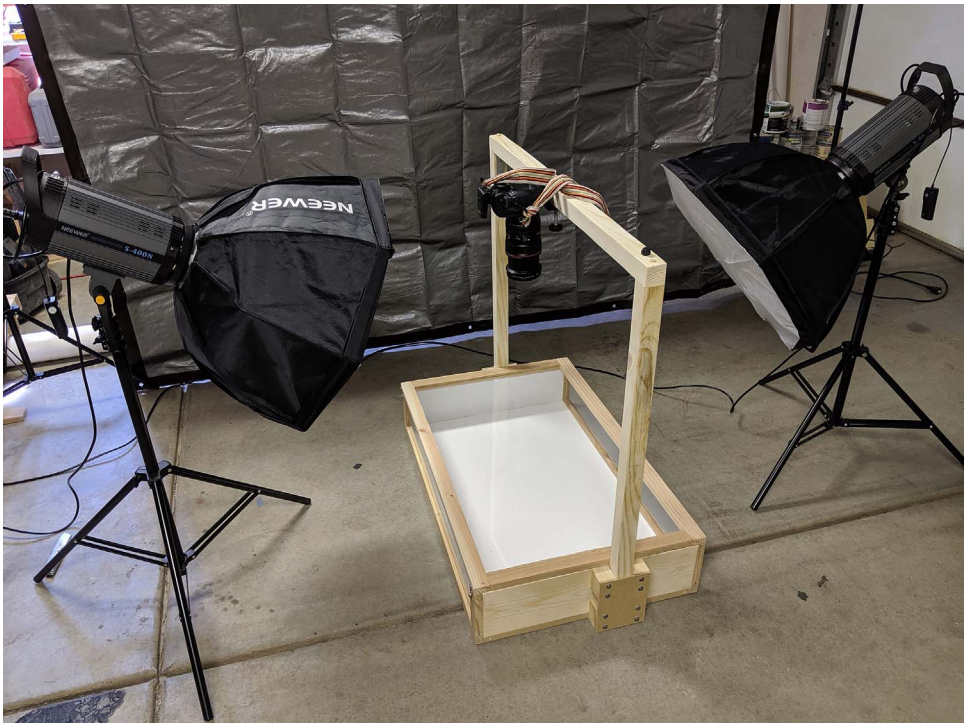
Fig. 4. Home-built lightbox/stage lighting kit with synchronized strobes and mounted camera.
